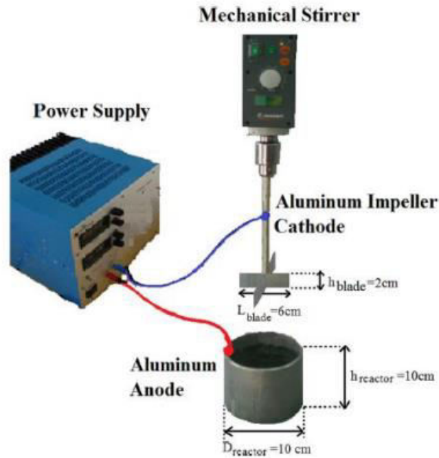
[Fig.2.3: Batch cylindrical reactor with rotating cathode electrode (Un et al., 2013)]
